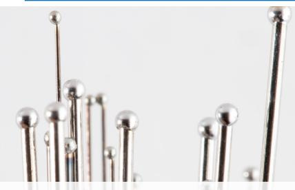
Beaded Wire System (BWS™) is a repeatable and controlled process for creating a homogenous, undifferentiated spherical bead at the end of a wire, rod, or tube. The bead of this system provides a secure attachment point without the need to incorporate external hardware - eliminating undesirable weight or friction in a system. With precision tooling, the size of this beaded end can be accurately controlled to meet high tolerance requirements for a wide array of applications.
