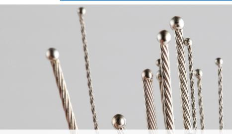
**Beaded Strand System (BSS™)** is a repeatable and controlled process for creating a homogenous, undifferentiated spherical bead at the end of a strand, cable, or wire rope. The bead of this system provides a secure attachment point without the need to incorporate external hardware - eliminating undesirable weight or friction in a system. With precision tooling, the size of this beaded end can be accurately controlled to meet high tolerance requirements for a wide array of applications.
