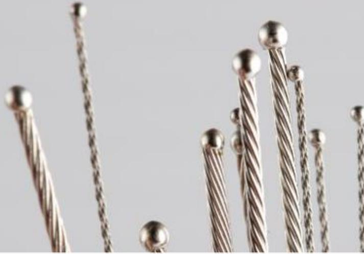
**Beaded Strand System (BSS™)** is a repeatable and controlled process for creating a homogenous, undifferentiated spherical bead at the end of a strand, cable, or wire rope. The bead of this system provides a secure attachment point without the need to incorporate external hardware - eliminating undesirable weight or friction in a system. With precision tooling, the size of this beaded end can be accurately controlled to meet high tolerance requirements for a wide array of applications.
